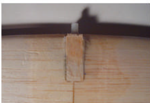
Wing Showing Torque Rod and Aileron Set-Up
